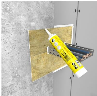
Fill all gaps > 10 mm with loose mineral fibre material, then with **HENSOMASTIK® 5 KS SP (Spachtel)** from both sides in full depth.
